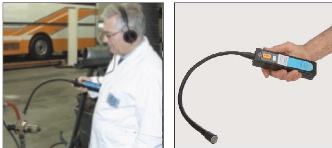
Above shows use of quality headphones and flexible pipe with sensor to get to a difficult spot to find an air leak.
